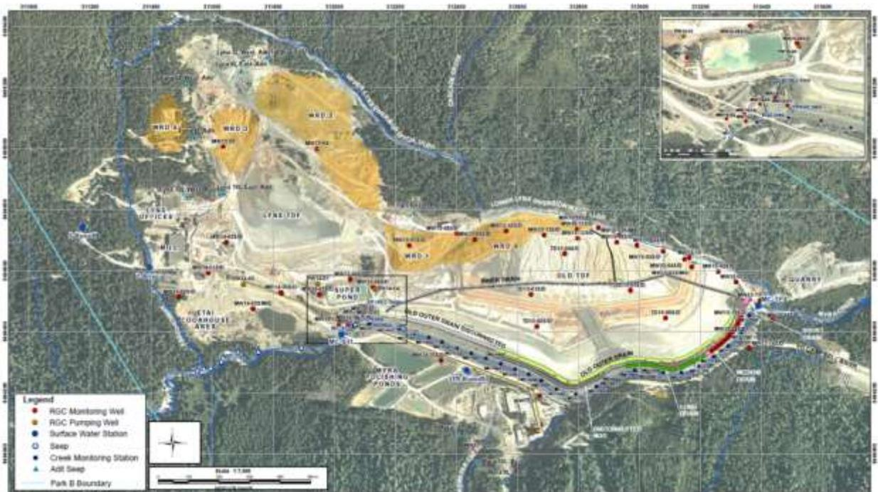
**Figure 1. General Mine Arrangement and Monitoring Locations, Nyrstar Myra Falls.**
